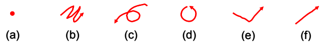
Figure 2: Pen gestures: (a) period (tap), (b) scratch-out, (c) roll, (d) small lasso, (e) span (perp), (f) flick.
