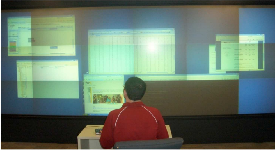
FIGURE 1. Processing desktop work on a wall-sized high-resolution display (size: 4.88 m wide x 1.83 m high, resolution: 6144 x 2034).
