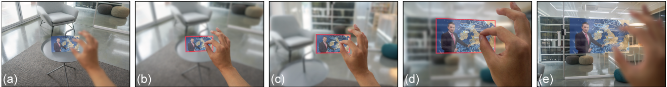
Figure 1. In a mock setup showing the flow of Projective Windows, (a) the user wishing to adjust the scale and position of an AR window (b) grabs the window, (c) moves it, (d) makes it bigger by bringing it closer, and (e) projects it to the desired position.
