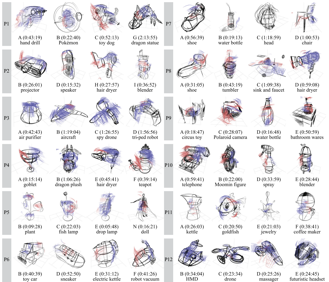
Figure 11. 3D design sketch outcomes produced by the participants using our workflow, and total time (h:mm:ss) taken.
