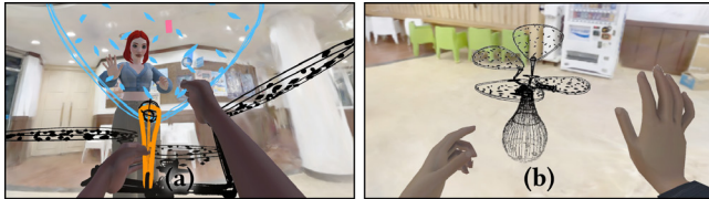
Figure 4: During VR acting, (a) one robot designer invisibly controls the robot, moving and rotating parts using bimanual grab gestures, (b) while another designer immersively experiences the robot’s services.
