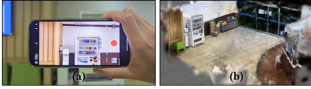
Figure 2: During workspace building, the robot designer (a) observes a site and records a video, and (b) produces a 3D Gaussian Splatting (3DGS) model of the environment.
